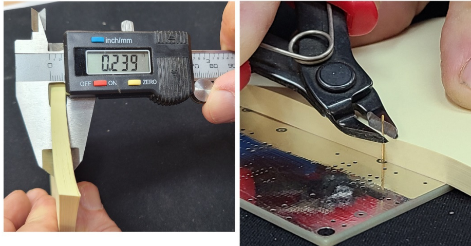
Figure 9 – Cutting Mill-Max pins to length using Post-It spacer
