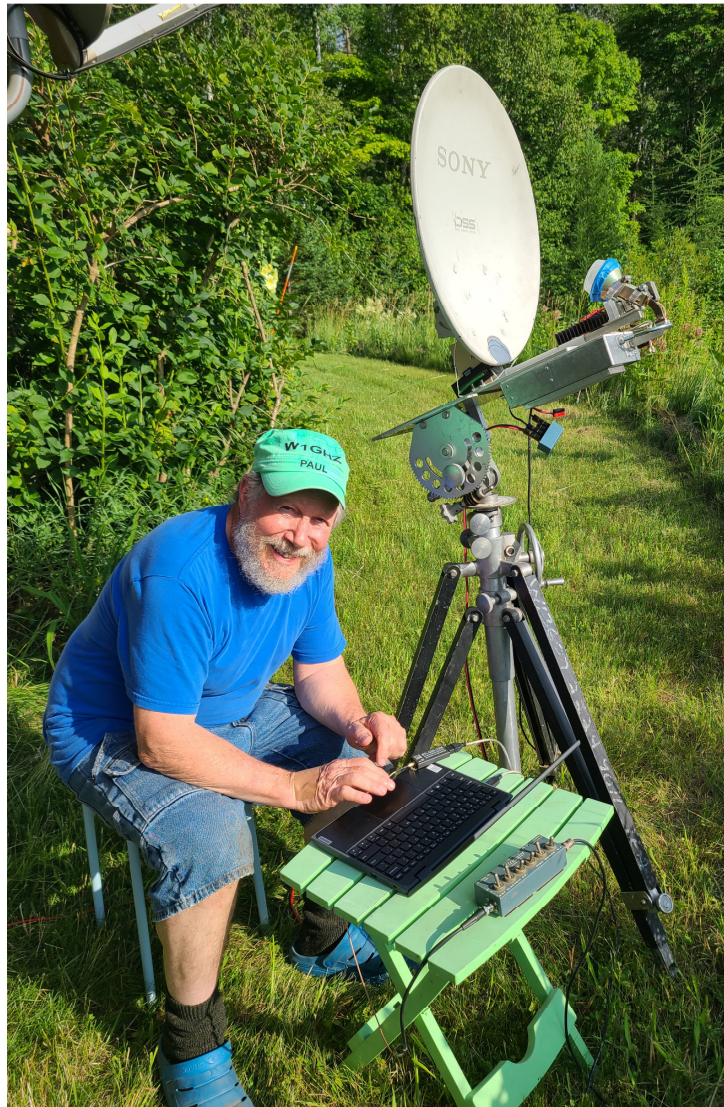
Figure 3 – Measuring sun noise of 10 GHz rover system
