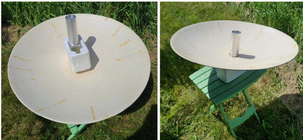
Figure 1 – Measuring sun noise – feedhorn shielded by dish from ground noise
