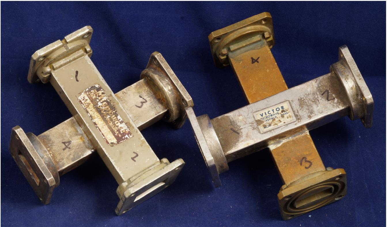
**Figure 13 - Round hole cross-guide directional couplers for 10 GHz in WR-90 waveguide**
