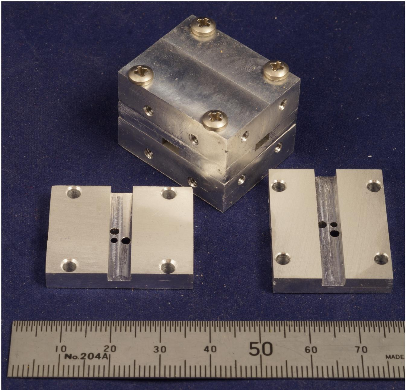
**Figure 10 - Machined round hole cross-guide 20 dB directional coupler for 47 GHz in WR-19 waveguide**
