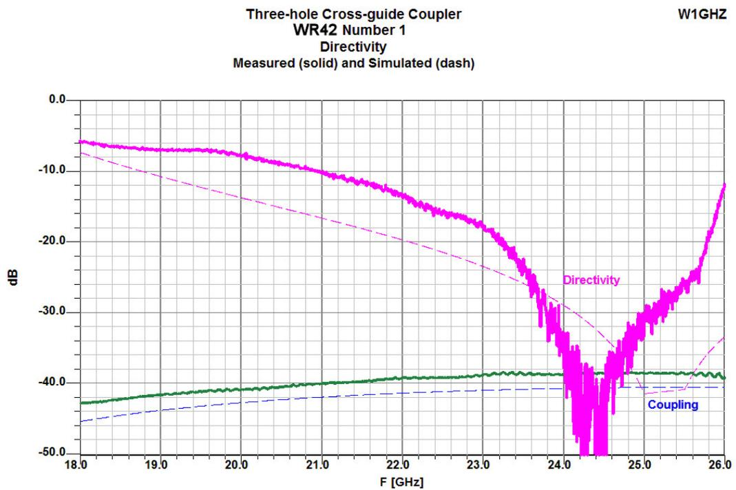
**Figure 8 - Measured performance comparison to simulation of round hole cross-guide 40 dB directional coupler for 24 GHz in WR-42 waveguide**
