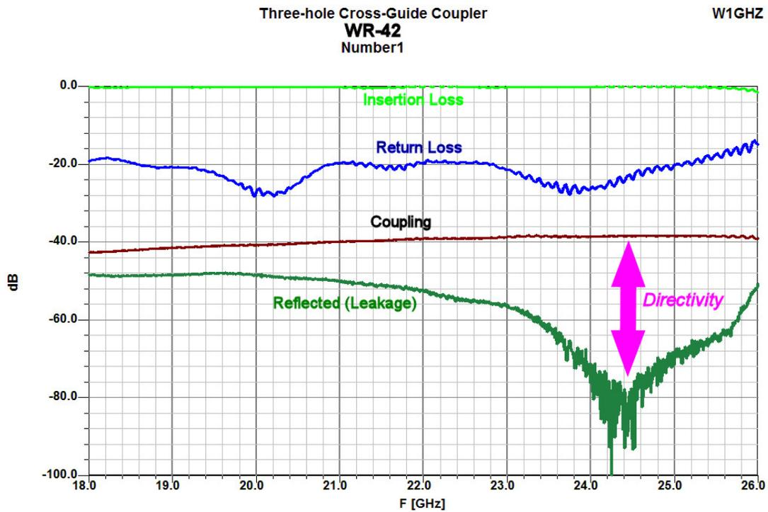
**Figure 7 – Measured performance of round hole cross-guide 40 dB directional coupler for 24 GHz in WR-42 waveguide**
