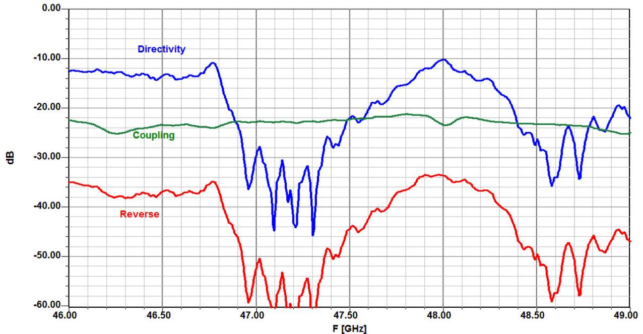
**Figure 11 - Measured performance of round hole cross-guide 20 dB directional coupler for 47 GHz in WR-19 waveguide**
