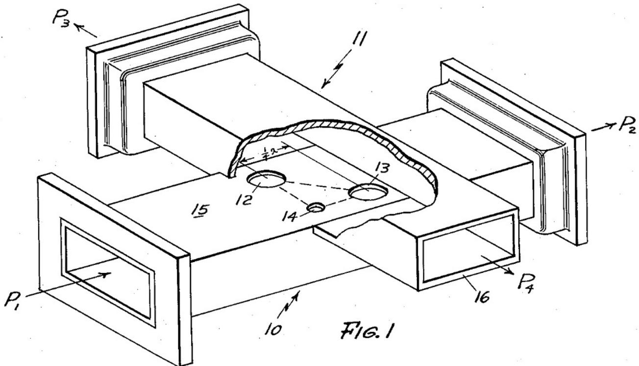
Figure 4 – Round hole cross-guide directional coupler sketch
