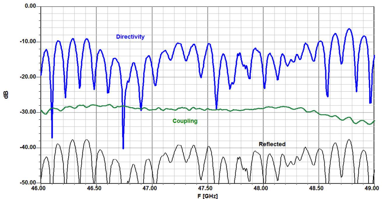
**Figure 9 - Measured performance of round hole cross-guide 30 dB directional coupler for 47 GHz in WR-19 waveguide**
