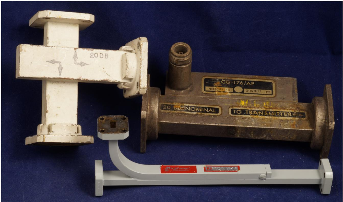
**Figure 2 – Surplus waveguide directional couplers. Clockwise from left: cross-guide coupler in WR-75, sidewall coupler in WR-90, and broadwall coupler in WR-28.**
