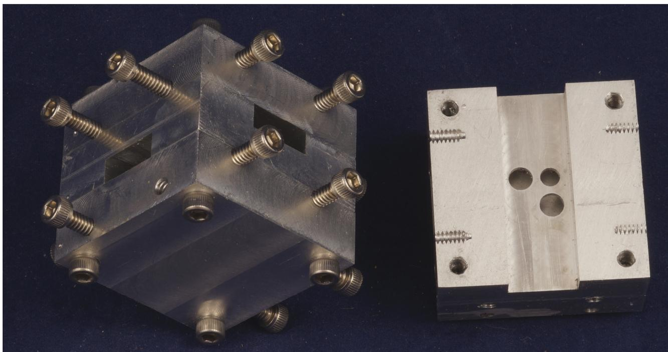
**Figure 6 – Machined round hole cross-guide coupler for 24 GHz in WR-42 waveguide**
