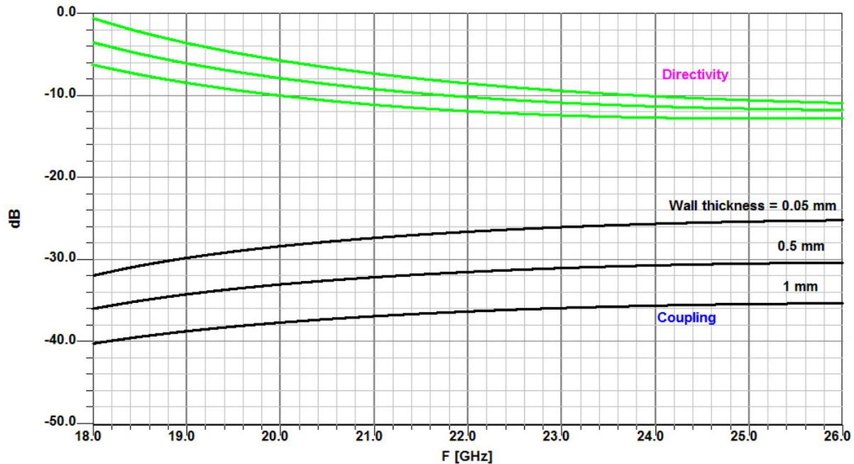
Figure 5 – Simulation of 30 dB round hole cross-guide directional coupler with dimensions from Wheeler graph
