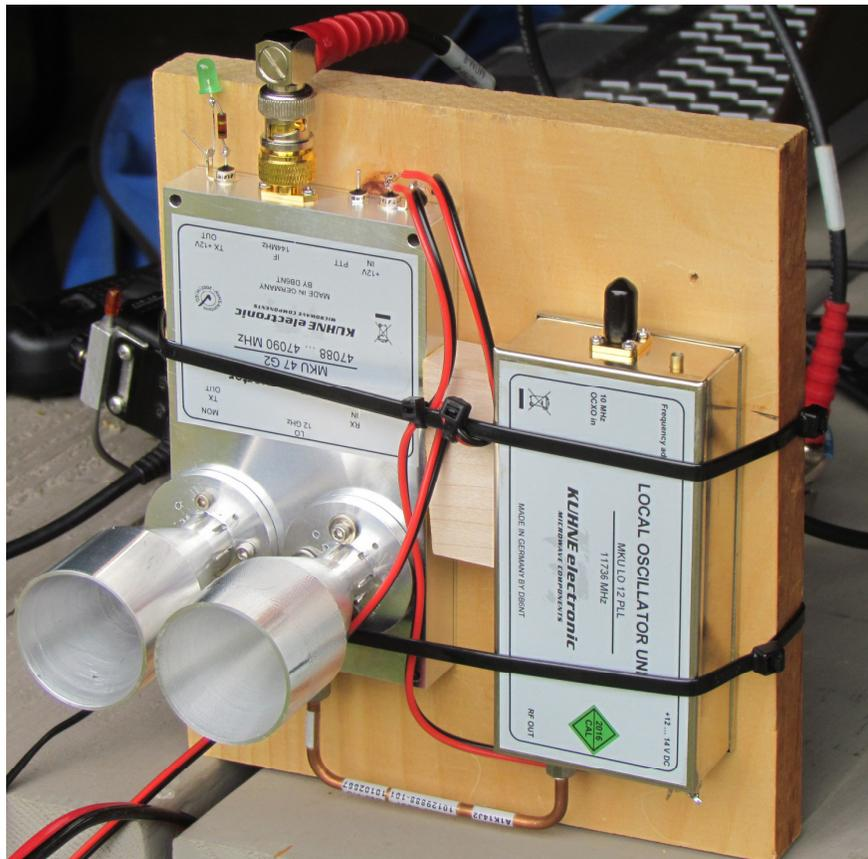
**Figure 1 – 47 GHz DB6NT Transverter breadboard with separate horns**
