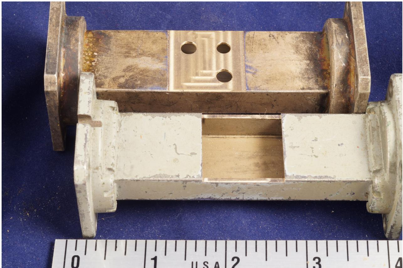
**Figure 12 - Round hole cross-guide directional coupler for 10 GHz in WR-90 waveguide fabrication from surplus waveguide before soldering together.**
