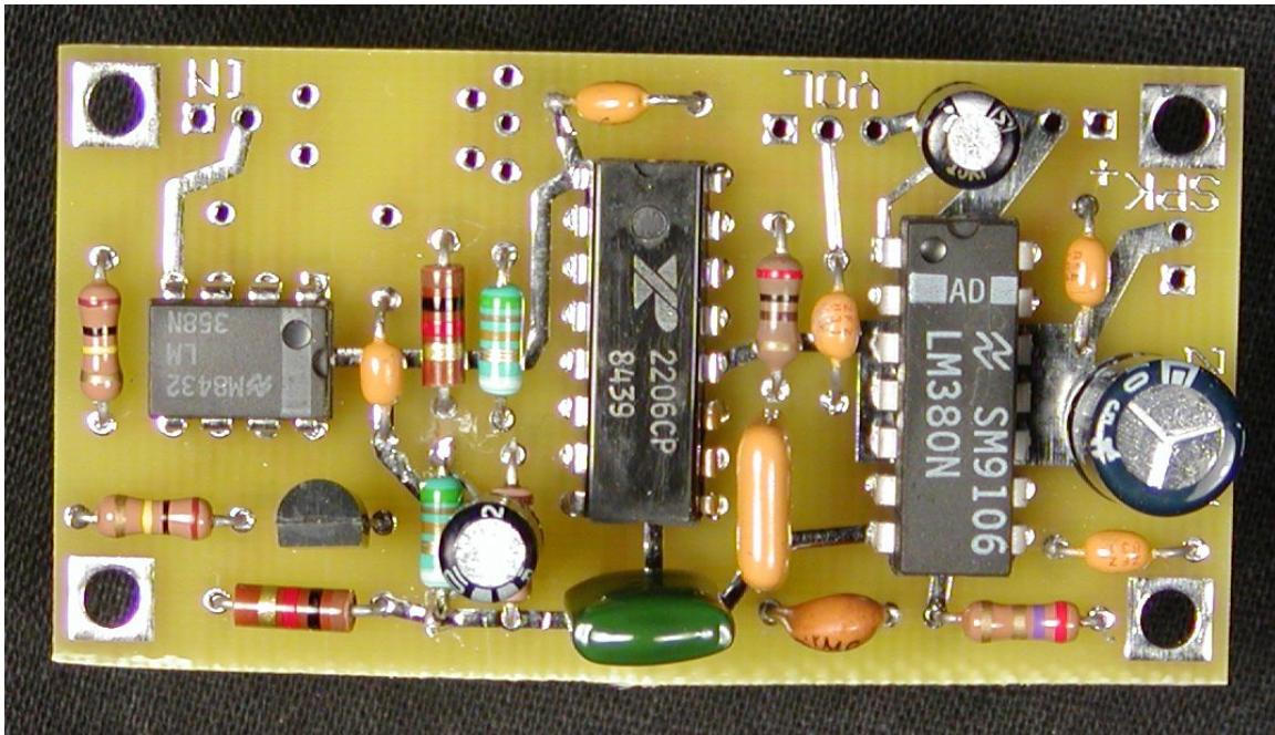
The final adjustment depends on the input. Many surplus test instruments have an output of 0 to 1 Volt for a chart recorder, while older tube instruments might have a 10-volt output. The 100K pot at the input is adjusted to provide a good pitch for a full-scale reading on the test meter, so that the output goes from a low growl at zero reading to that pitch at full scale, allowing peaking by ear.
