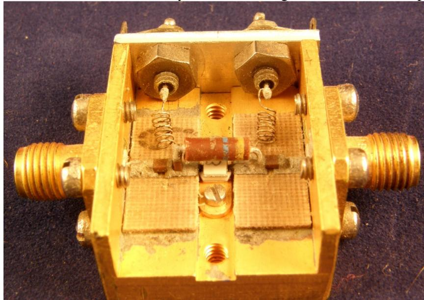
*Figure 5 – Broadband feedback amplifier using 1/2 watt GaAsFET*
