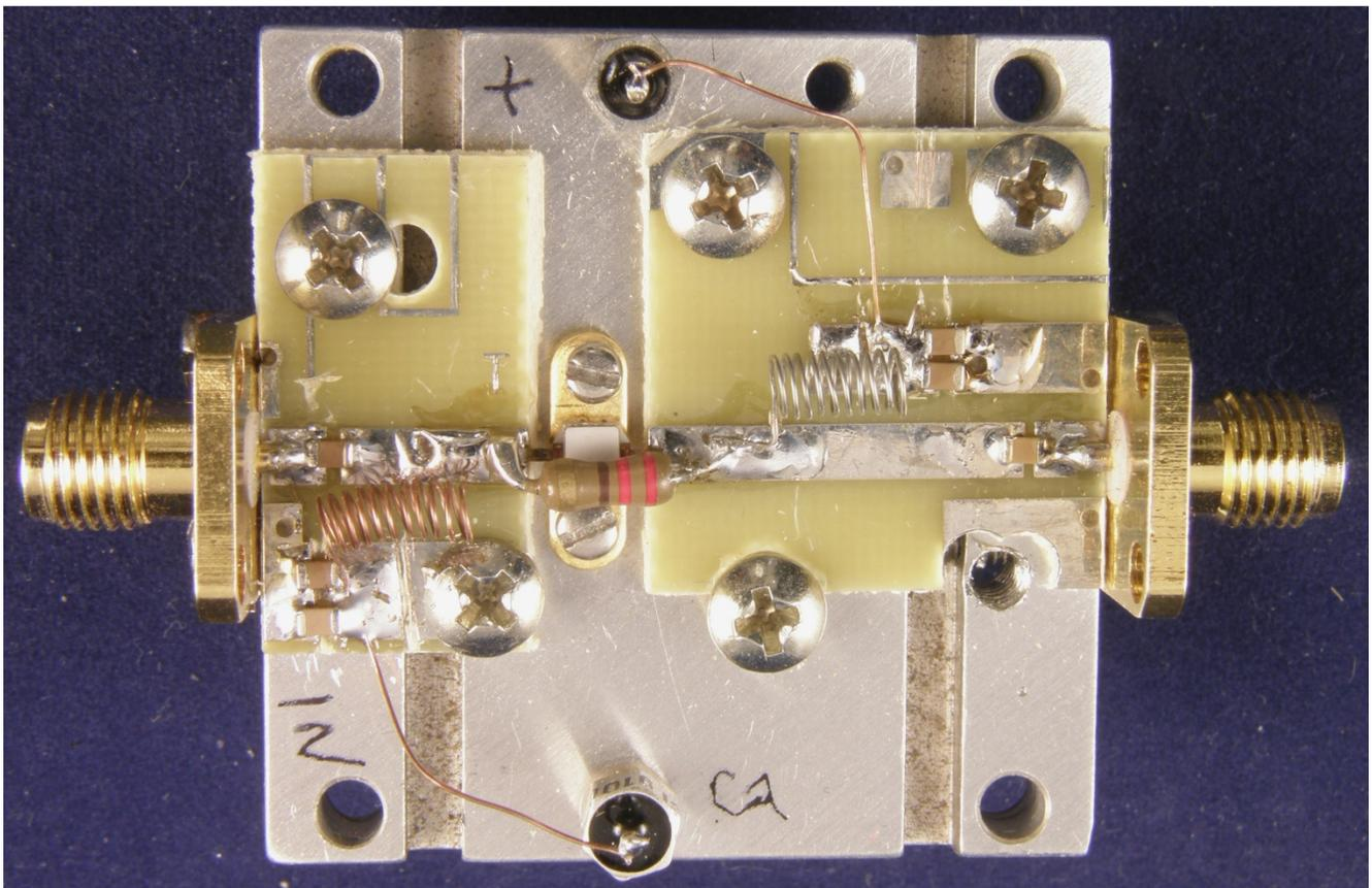
*Figure 6 – Broadband feedback amplifier using ½ watt GaAsFET*
