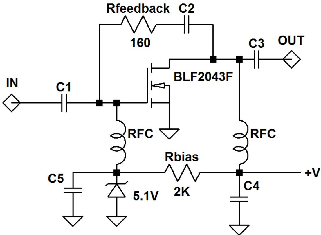
Figure 3- Schematic of BLF2043F Broadband Amplifier
