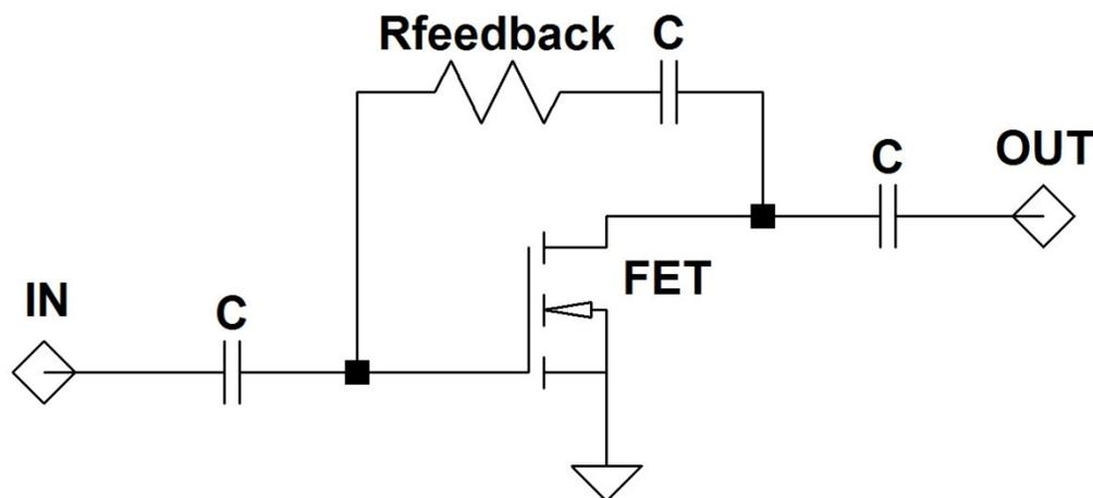
Figure 1- Schematic of FET Broadband Feedback Amplifier
