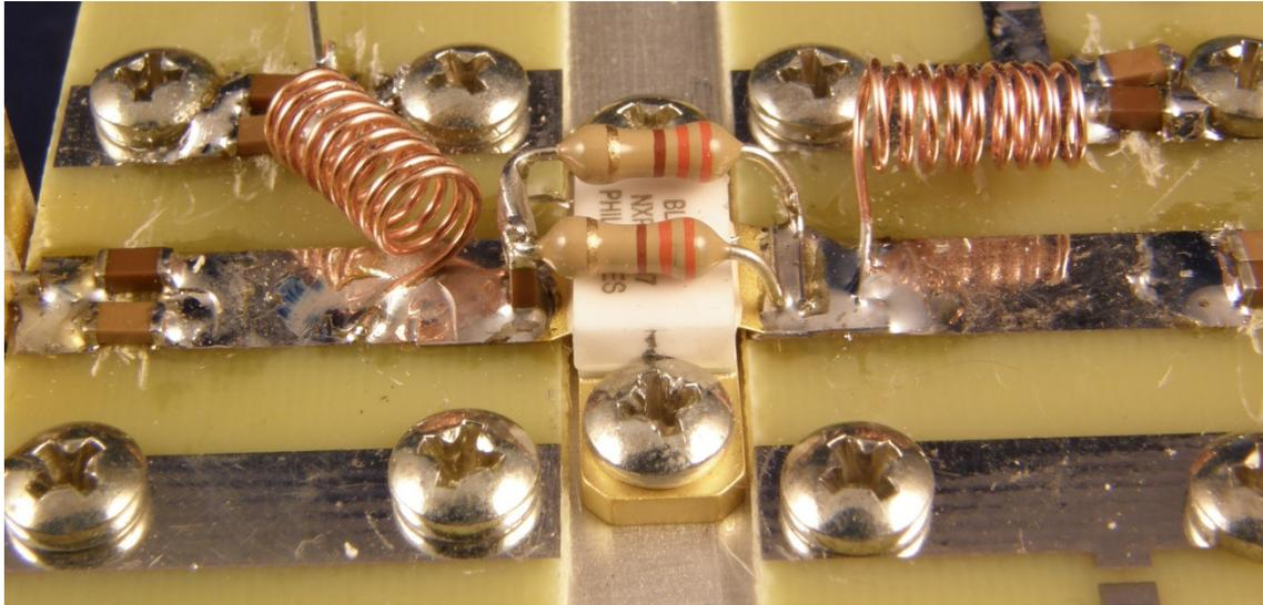
*Figure 4 – Closeup of BLF2043F UHF Broadband Amplifier*
