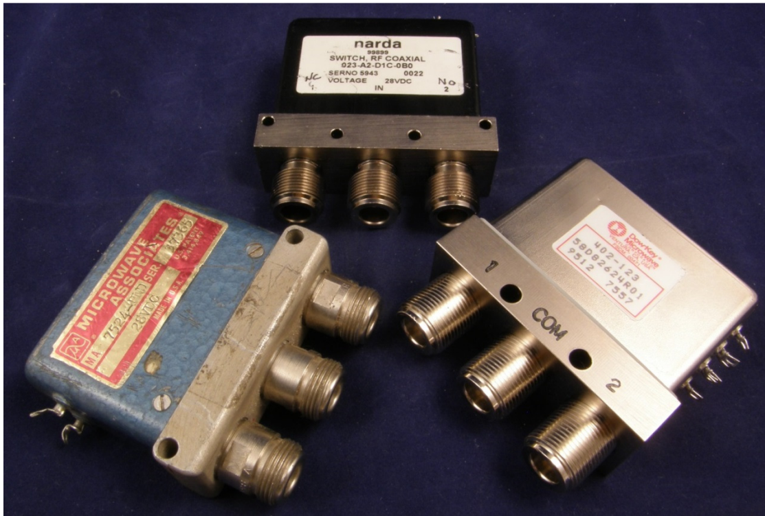
Figure 2 – Coax relays with good isolation at 1296 MHz
