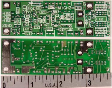
A photograph of a completed sequencer is shown in Figure 5. Construction is straightforward with common thru-hole components, and assembly goes pretty quickly. The LEDs are shown mounted on the board, but you'll probably want them mounted to the box for visibility, probably with an additional LED to show that the power is on. My station sort of evolved into using red for power, green for transmit, and yellow or blue for other things, but you might choose different colors.
