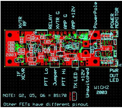
PowerPole<sup>5</sup> connector for the power input in the layout, so that the sequencer can be mounted on the panel as the power connector for the complete rig. The final fail-safe is the idiot diode, D9, to protect against reversed polarity – it will blow the fuse, so make sure there is a fuse in the power lead! The layout and
