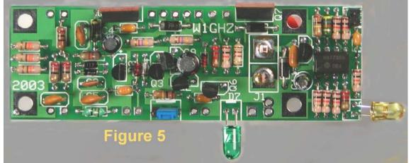
Assembly order isn't critical. I usually start with the PowerPoles, then resistors in order (R1, R2, etc.), then capacitors, followed by diodes, then transistors and the remainder. Soldering and lead trimming is in groups so there aren't too many leads in the way. All the components are on the top side, so soldering is on the bottom except for the PowerPoles. The boards are soldermasked to help prevent solder bridges causing unwanted shorts.
