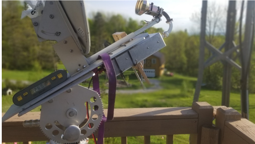
Figure 7 – Measuring sun noise and calibrating elevation tilt
