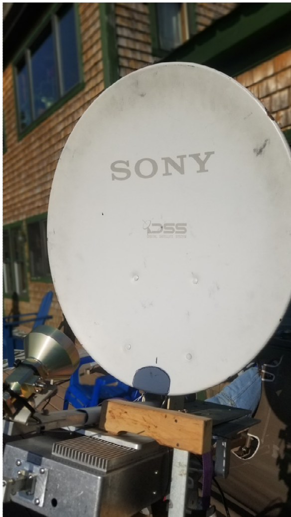
Figure 7 – Measuring sun noise and calibrating elevation tilt
