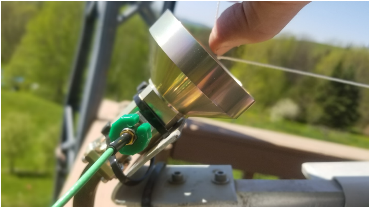
Figure 5 – Using modified string lengths to align feed at center of aperture
