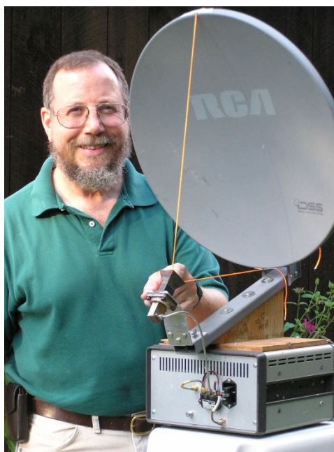
Figure 2 – Finding dish focus using string method
