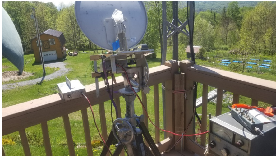
Figure 6 – Slant antenna range for testing tilt alignment on the two bands
