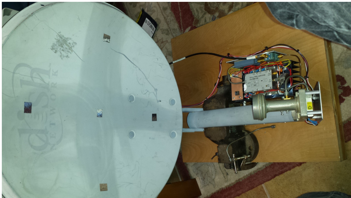
Figure A5: 10 GHz transverter interior. The filter is in the lower center. The phase lock is the aluminum box in the upper center. The YIG is just to the right of the phase lock box.
