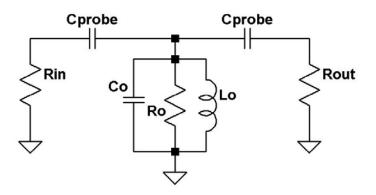
Figure 4. Pipe-cap resonator equivalent circuit
