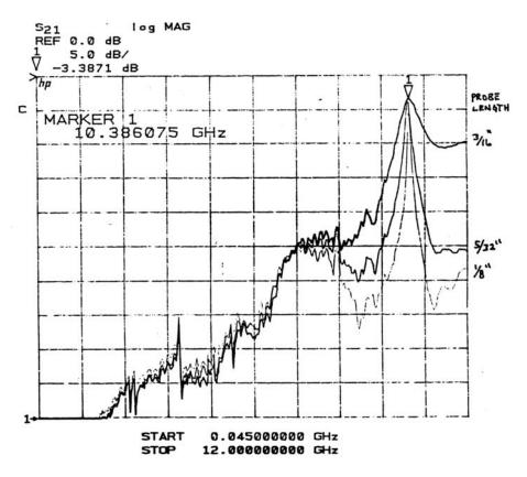
Figure 14. Measured response of 1/2" pipe-cap filter
