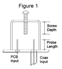
tuning screw acts as the coax center conductor, with a radial electric field around it; the field intensity increases toward the open end of the screw. The resonant frequency is determined by the inserted length of the screw; Figure 3 shows that the same screw length produces the same resonant frequency in three different sizes of pipe caps. The other dimensions do not affect the frequency, as they would if a waveguide cavity mode were involved.
