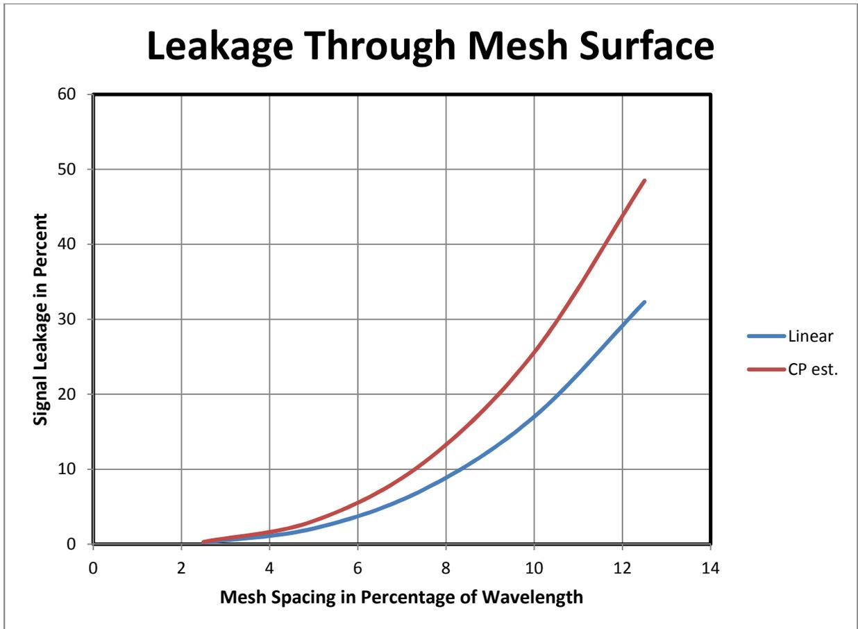
**Figure 12 – Leakage through wire mesh reflector based on Otoshi**
