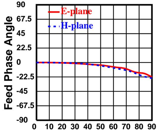
Dish diameter =  $20\lambda$  Feed diameter =  $1.7\lambda$
