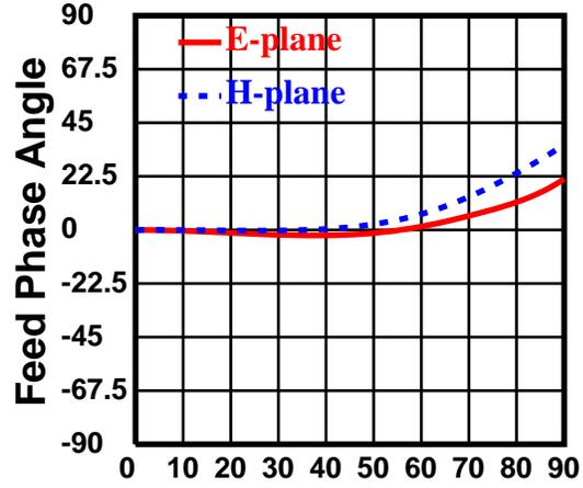
Dish diameter =  $20 \lambda$  Feed diameter =  $1.9 \lambda$
