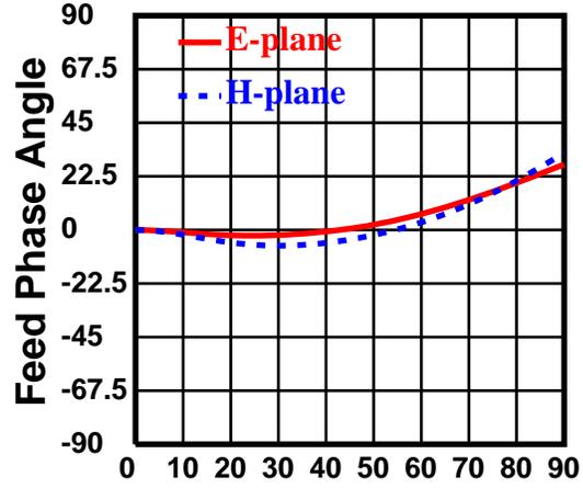
Dish diameter =  $20 \lambda$     Feed diameter =  $2.1 \lambda$
