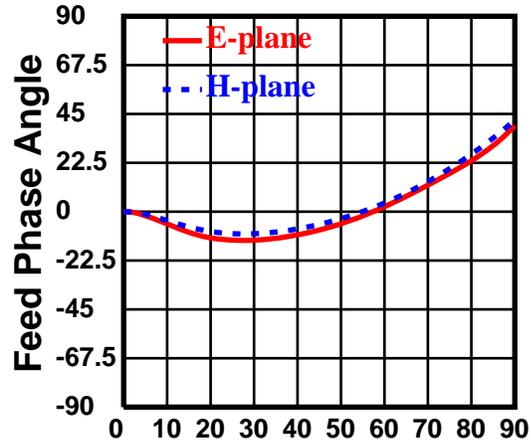
Dish diameter =  $20\lambda$  Feed diameter =  $1.9\lambda$
