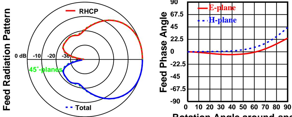
Dish diameter =  $27\lambda$  Feed diameter =  $2.26\lambda$  Rotation Angle around specified Phase Center =  $0.186\lambda$  inside aperture
