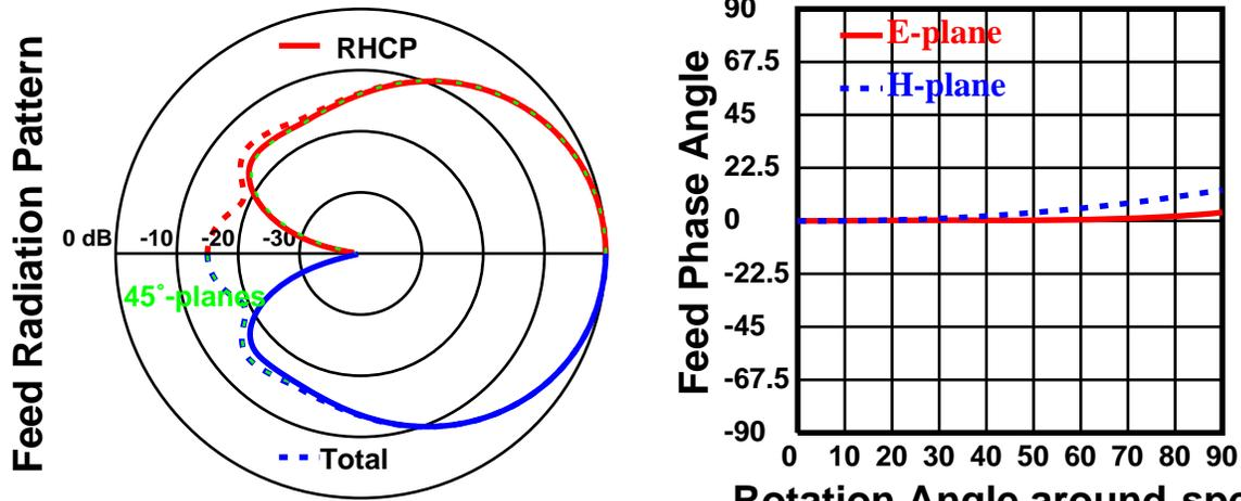
Dish diameter =  $20 \lambda$     Feed diameter =  $0.7 \lambda$
