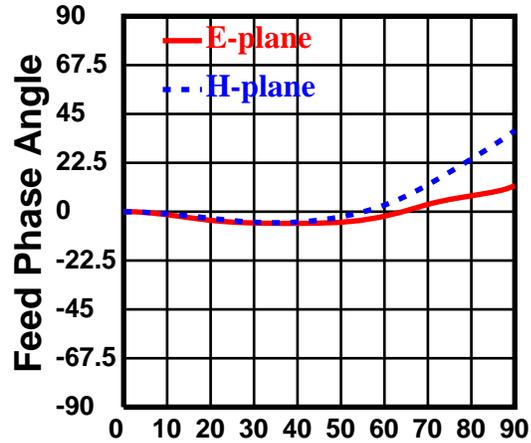
Dish diameter =  $20\lambda$  Feed diameter =  $1.7\lambda$
