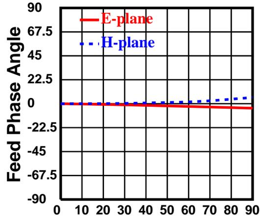
Dish diameter =  $20 \lambda$  Feed diameter =  $1 \lambda$
