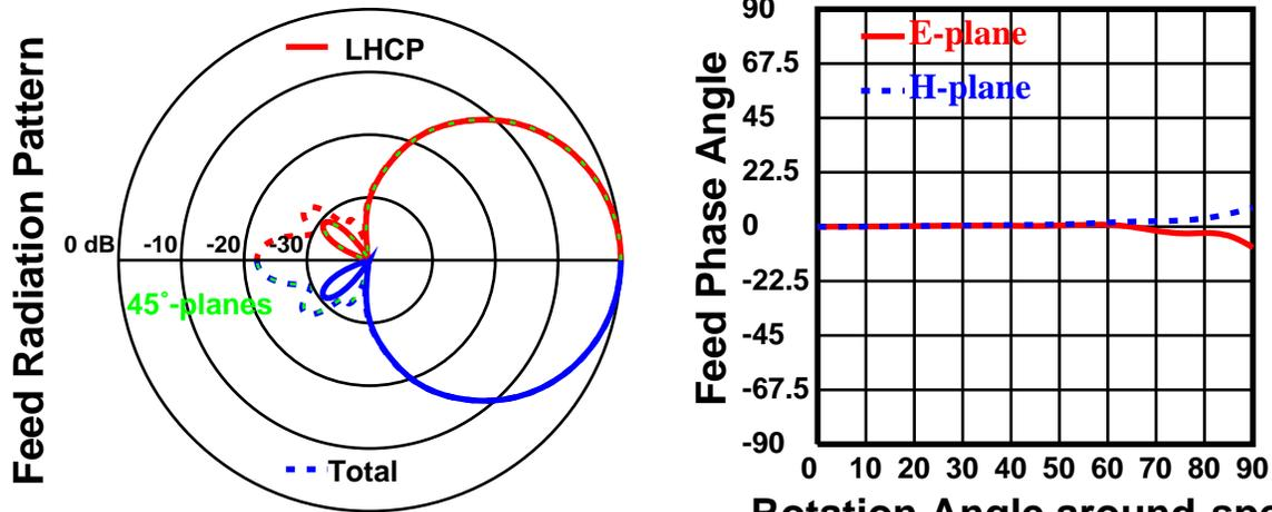
Dish diameter =  $20\lambda$     Feed diameter =  $1.22\lambda$
