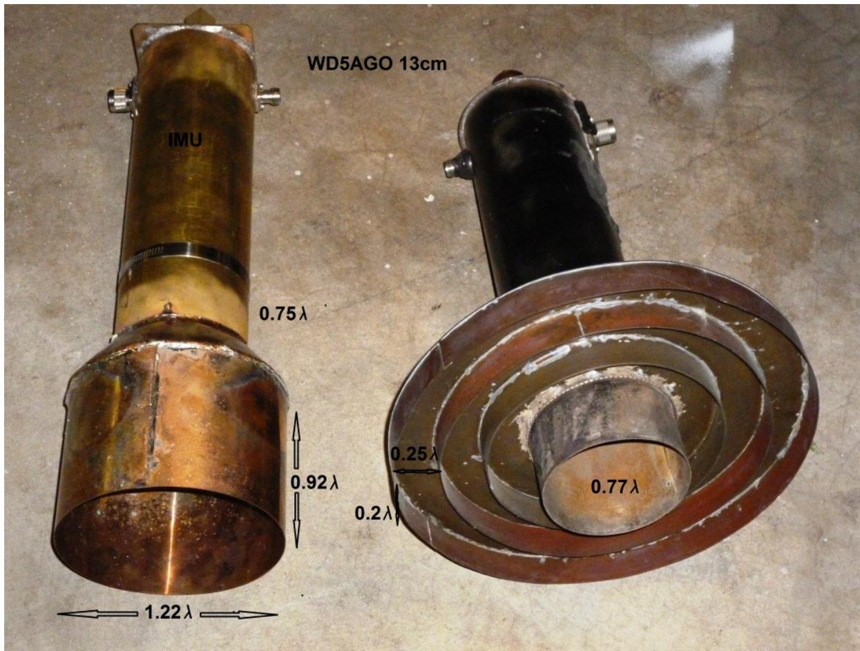
**Figure 9 – Feedhorns for 13 cm fabricated and measured by WD5AGO**
