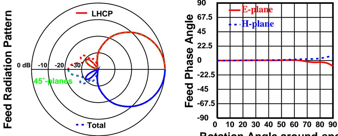
Dish diameter =  $27\lambda$  Feed diameter =  $1.22\lambda$
