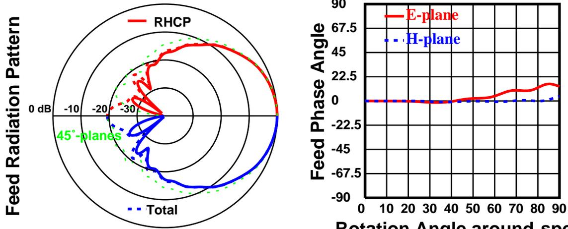
Dish diameter =  $20\lambda$  Feed diameter =  $1.5\lambda$
