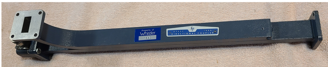
Figure 19 – HP X752c waveguide directional coupler with high directivity
