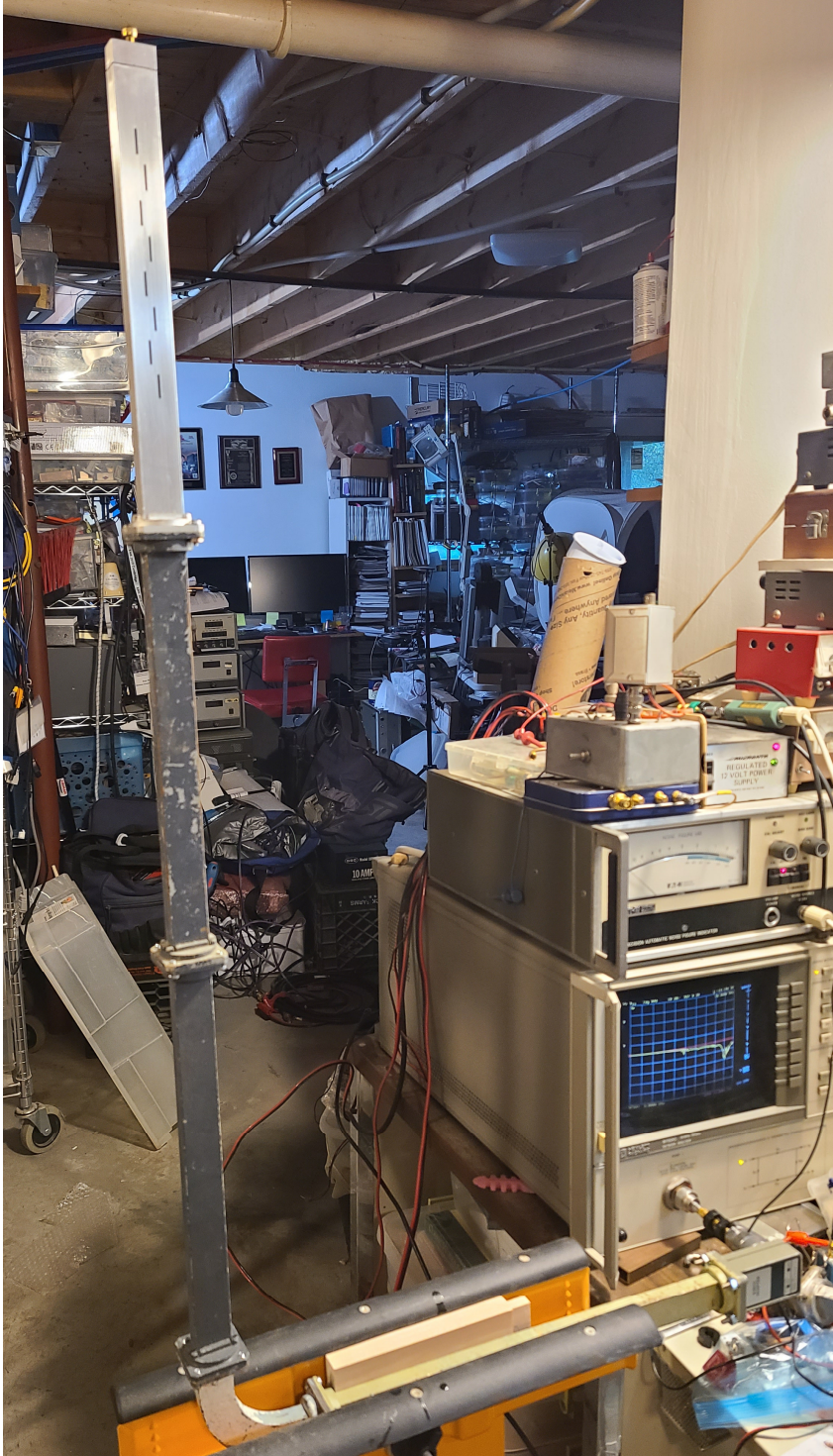
Figure 17 – Elevating the slot antenna high enough to tune
