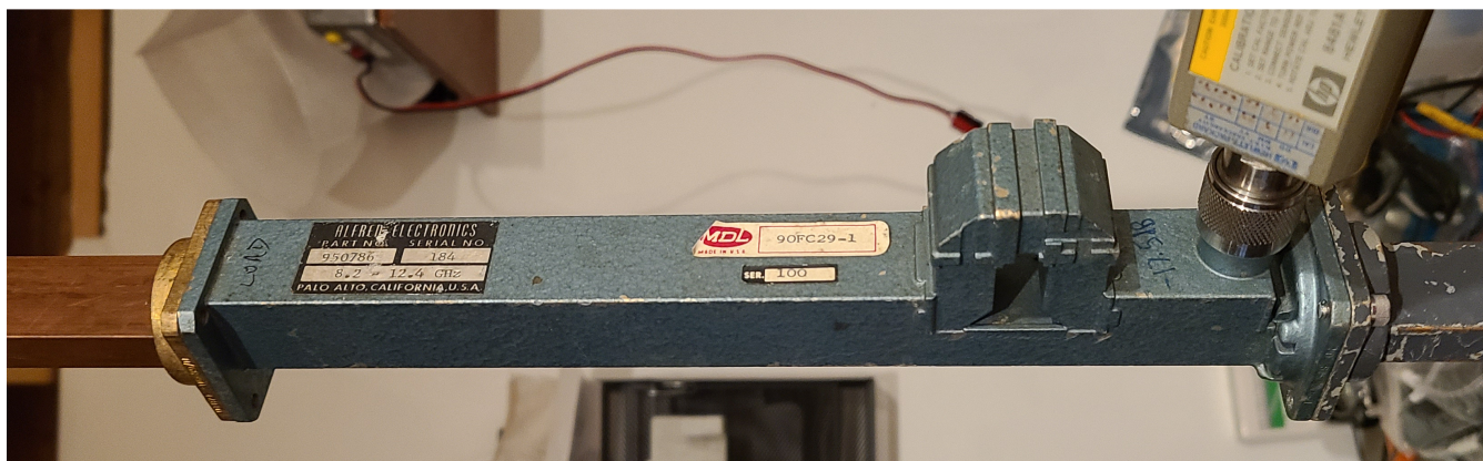
Figure 18 – Alfred Electronics X-band directional coupler with high directivity
