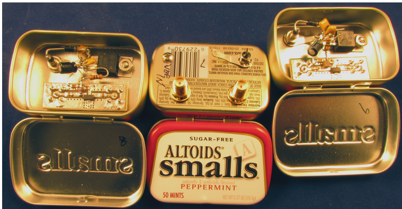
Figure 1- MMIC preamps in Altoids tins
