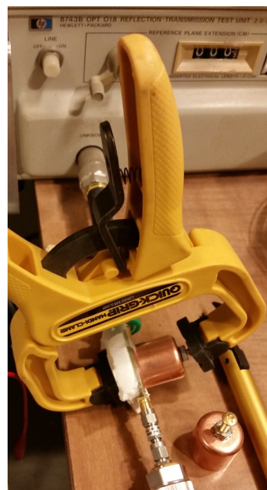
Figure 6 – Pipe-cap filter testing
